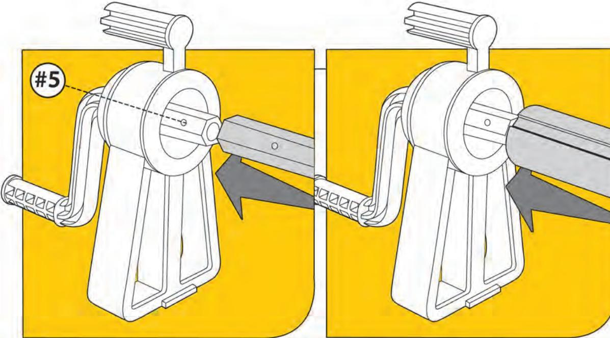
Insert tubes D into tubes E. Slide them together until the 2 supports rest across the surrounds of the pool. Make sure that tube E is exactly centred and that Z1 and Z2 are equal. Also make sure that a minimum (1-1/2") part of the tube is covered by the central tube.
