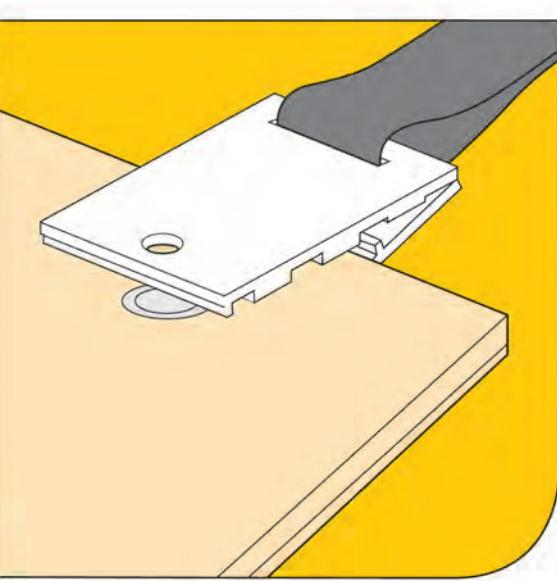
Position the cover over the pool and clip it as shown in the drawing. Tie the clips #12 at the same distances as the Velcro stuck on the tubes. Make sure that the lengths of the belts allow the cover to remain flat over the pool in order to impede wind entering under the cover.
