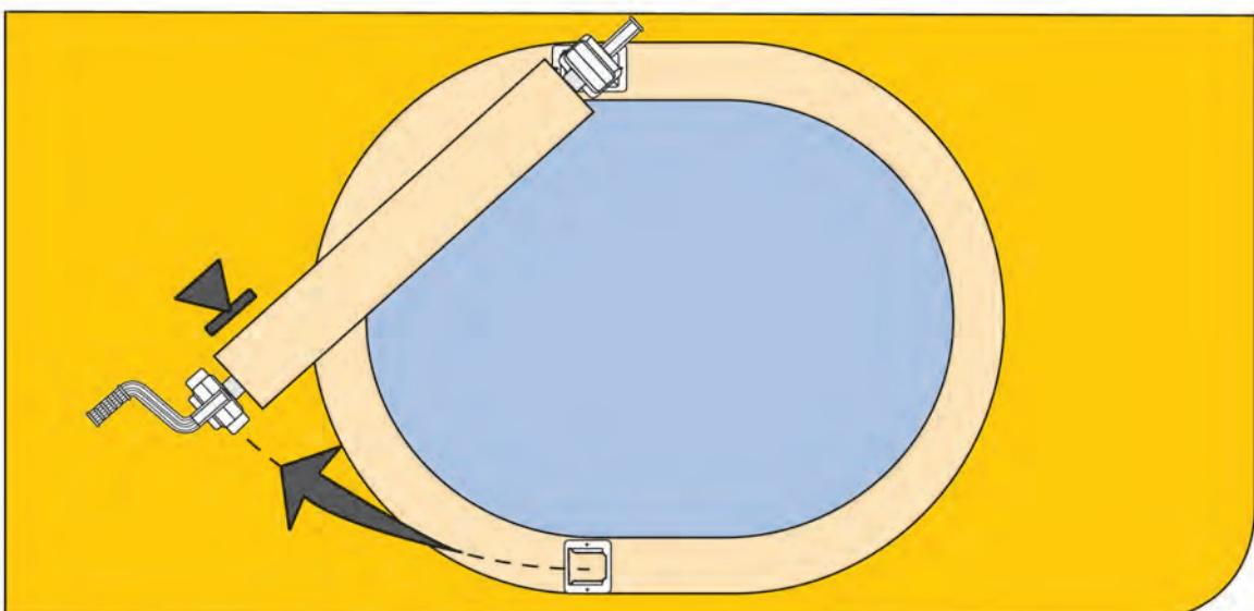
To remove the roller pull support #1 and the crank-arm of its base, around the pool. Check that support #2, rests on the surrounding of the pool or completely remove it.
