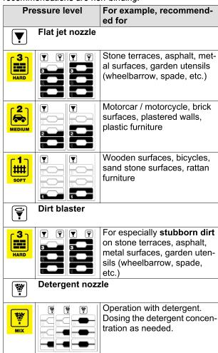
**Note:** When working with T-Racers and other accessories, the pressure indicator is not indicative. So that correct function is guaranteed, always set the pressure on the high-pressure gun to the highest level. Make any possible adjustments directly on the accessories.
